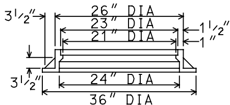
SECTION A-A GRAY IRON CAST FRAME WT. 390 LBS.
